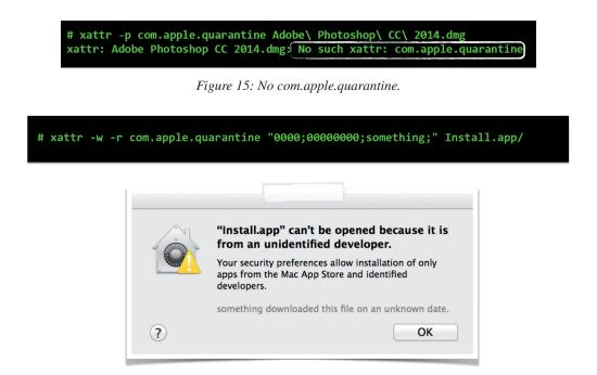
Figure 16: With the quarantine attribute set, Gatekeeper displays an alert.
