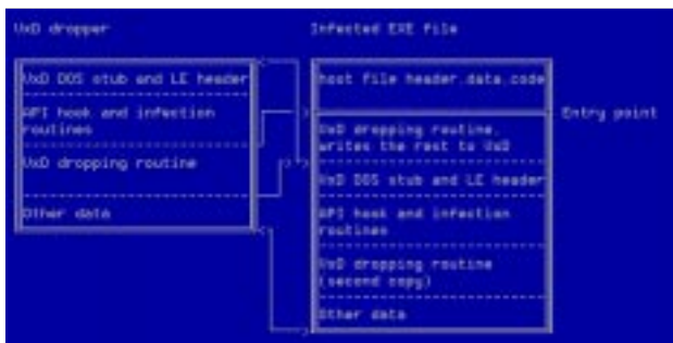
Figure 1: Punch exists in two forms; the VxD file version (found in VVFS.VXD) and the EXE file version.
