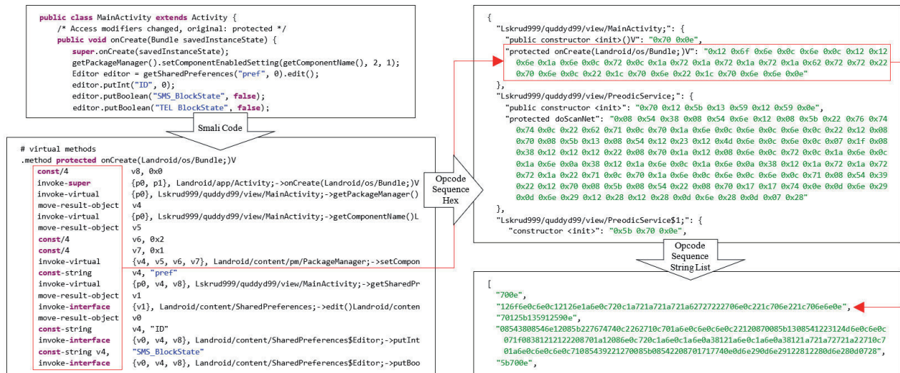
Figure 6: How to extract opcode sequence by method in classes.dex.
